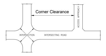
Figure 6. Corner Clearance Illustration
