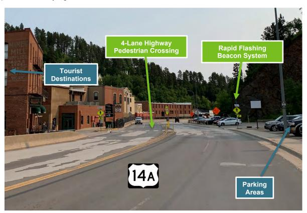
Figure 20. Crosswalk with Rapid Flashing Beacon across US14A at Wall Street
