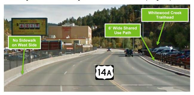
Figure 22. Shared Use Path Designation on US14A East Sidewalk (Facing North)
