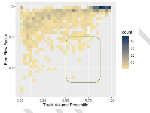
Figure 19: Free Flow Factor vs Truck Volumes on Roadway Segments
