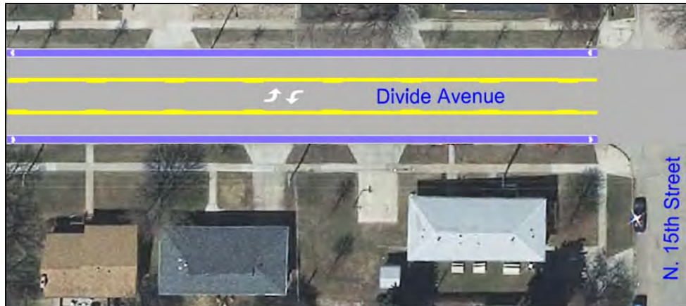
Figure 29. Example Implementation of 3-Lane Section with Bike Lanes on Divide Ave
