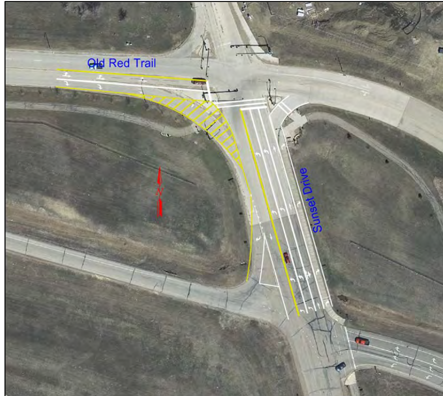
Figure 8. Lane Striping and Reconfiguration at Sunset Drive and Old Red Trail Intersection
