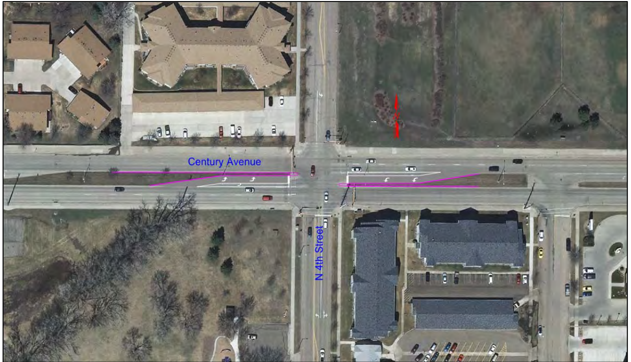
Figure 33. Left Turn Offsets at Intersection of 4th Street and Century Avenue Intersection
