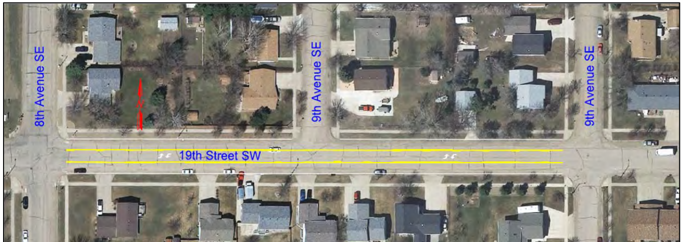
Figure 15. Example of Implementation of 3-Lane Section on 19 th Street
