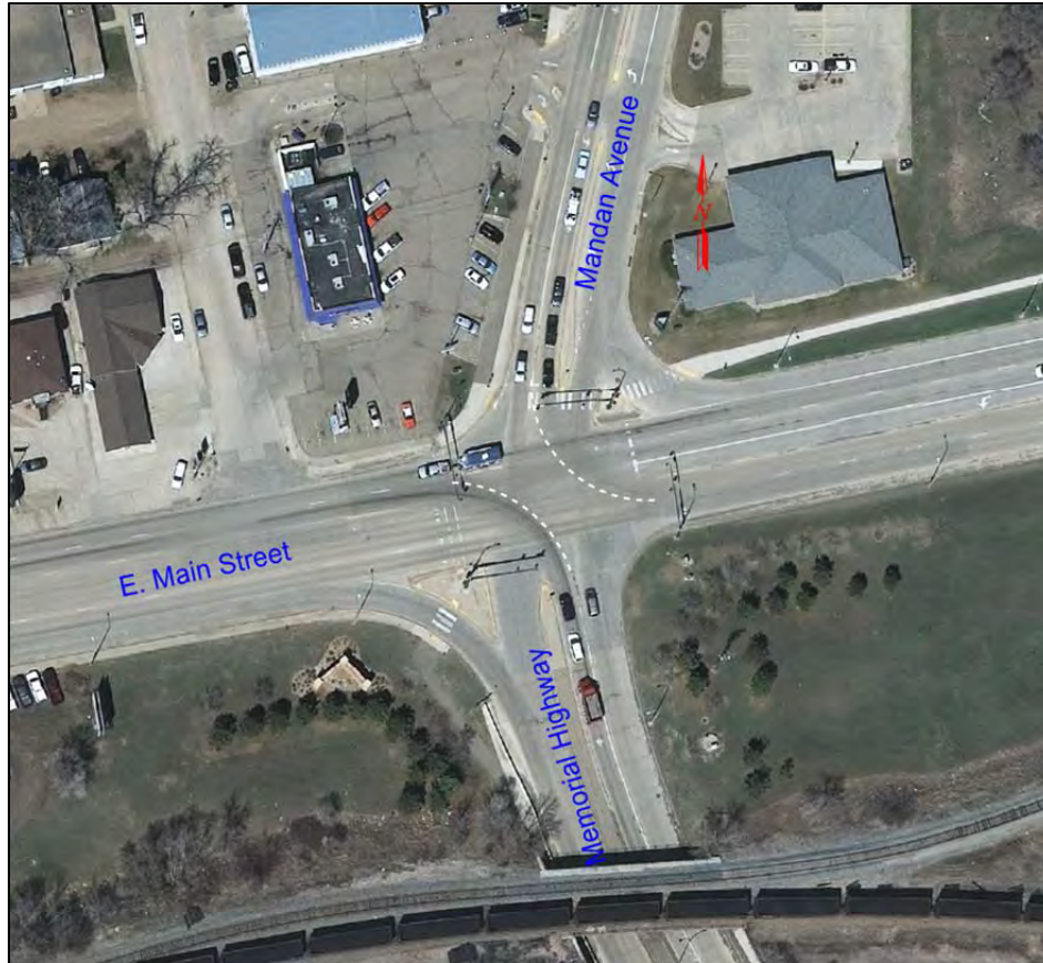
Figure 11. Intersection Guidance Striping at Mandan Avenue and Main Street Intersection
