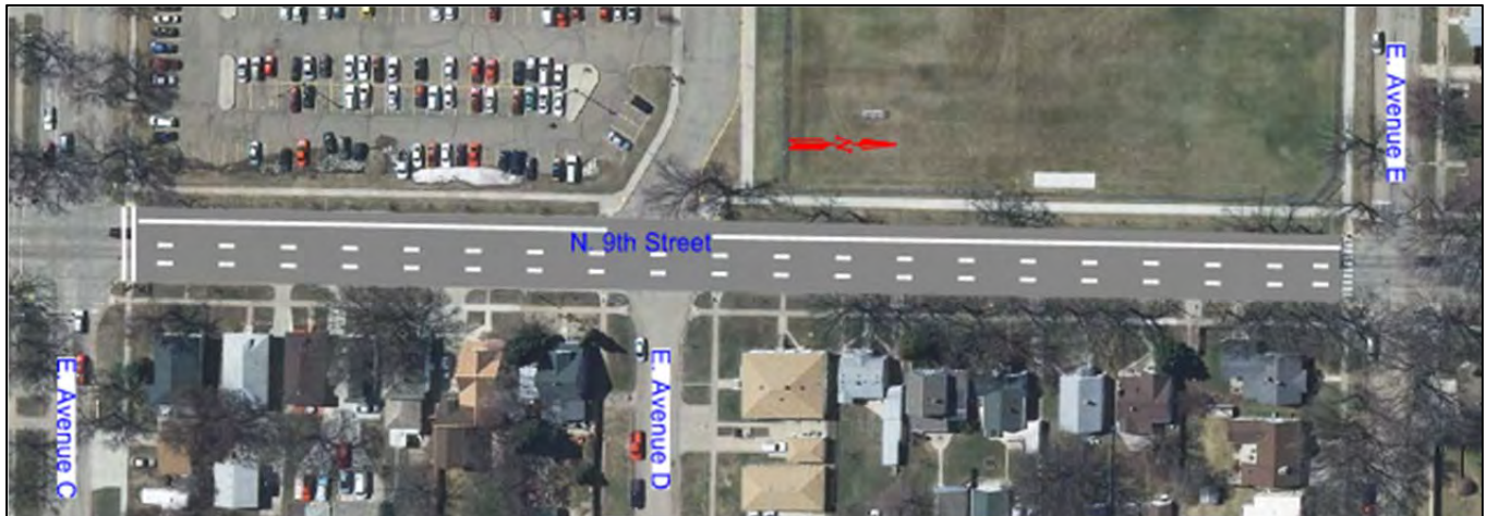
Figure 36. Example of Implementation of 3-Through Lane Section with Parking on 9th St
