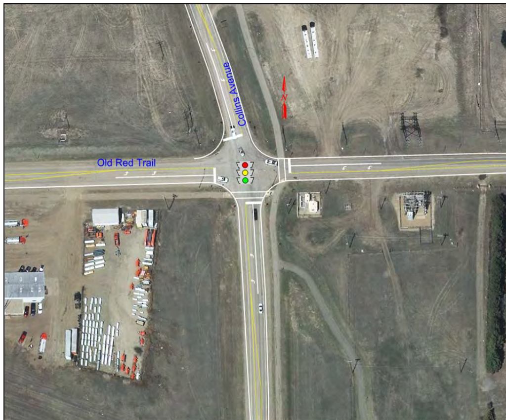
Figure 17. Lane Configuration and Possible Traffic Signal at Collins Avenue and Old Red Trail Intersection
