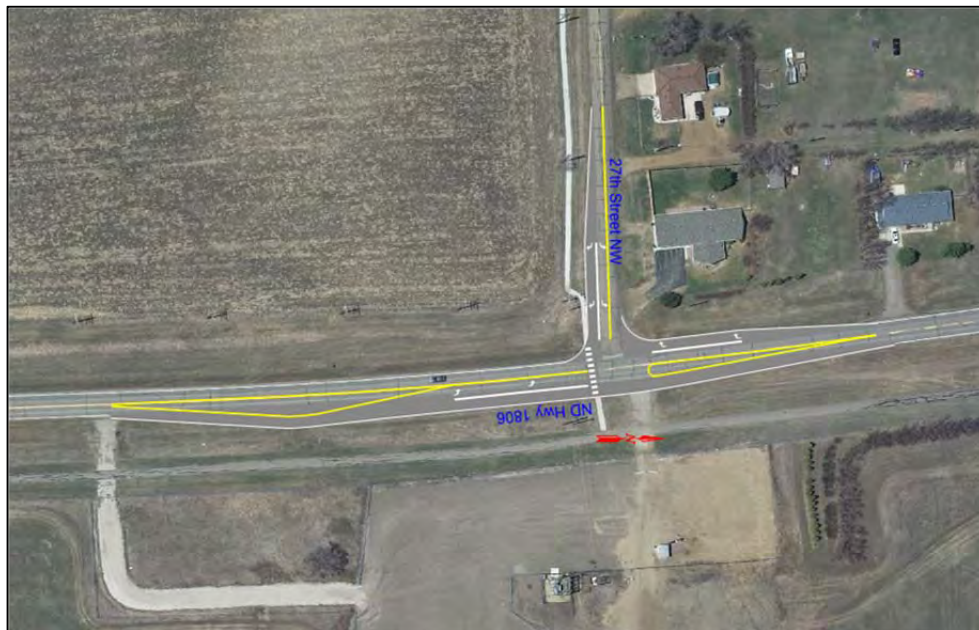
Figure 18. Turn Lanes on ND 1806N at 27 th St
