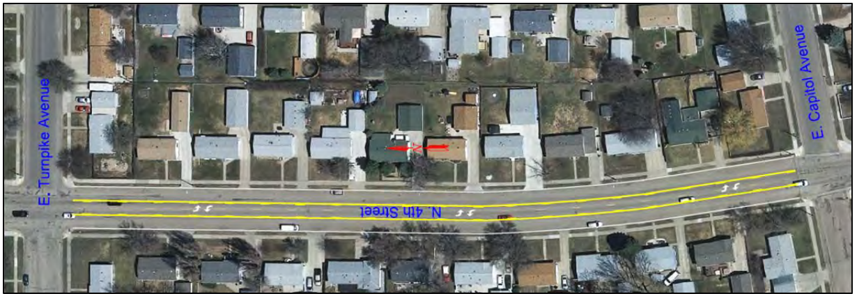
Figure 31. Example of Implementation of 3-Lane Section on 4th Street
