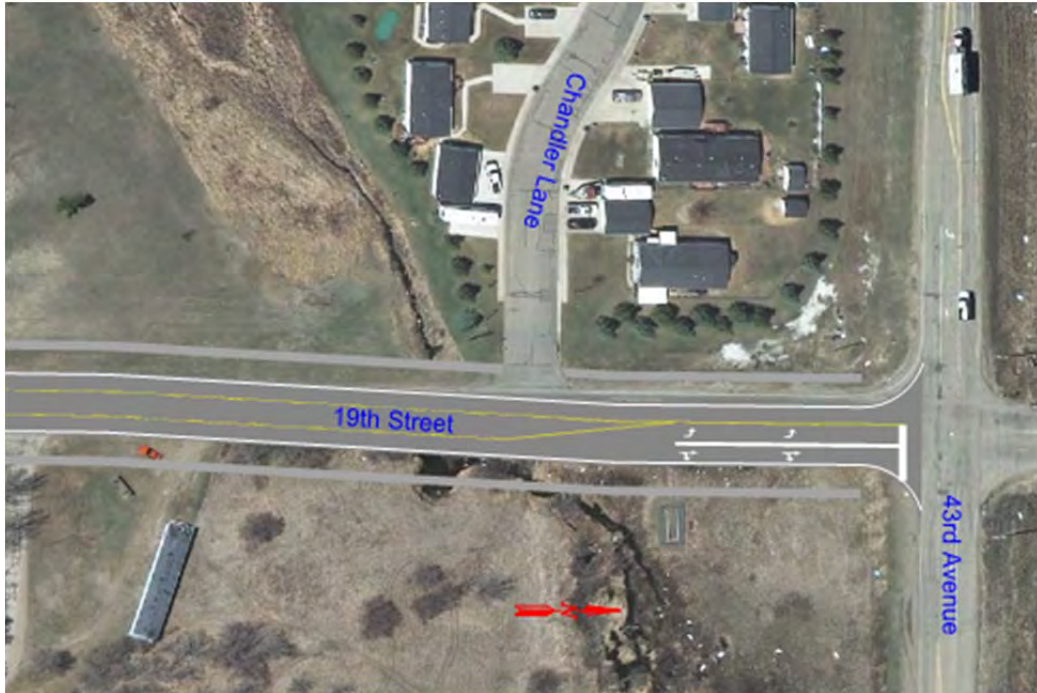
Figure 45. Turn Lane and Approach Realignment at 19th Street and 43rd Street Intersection
