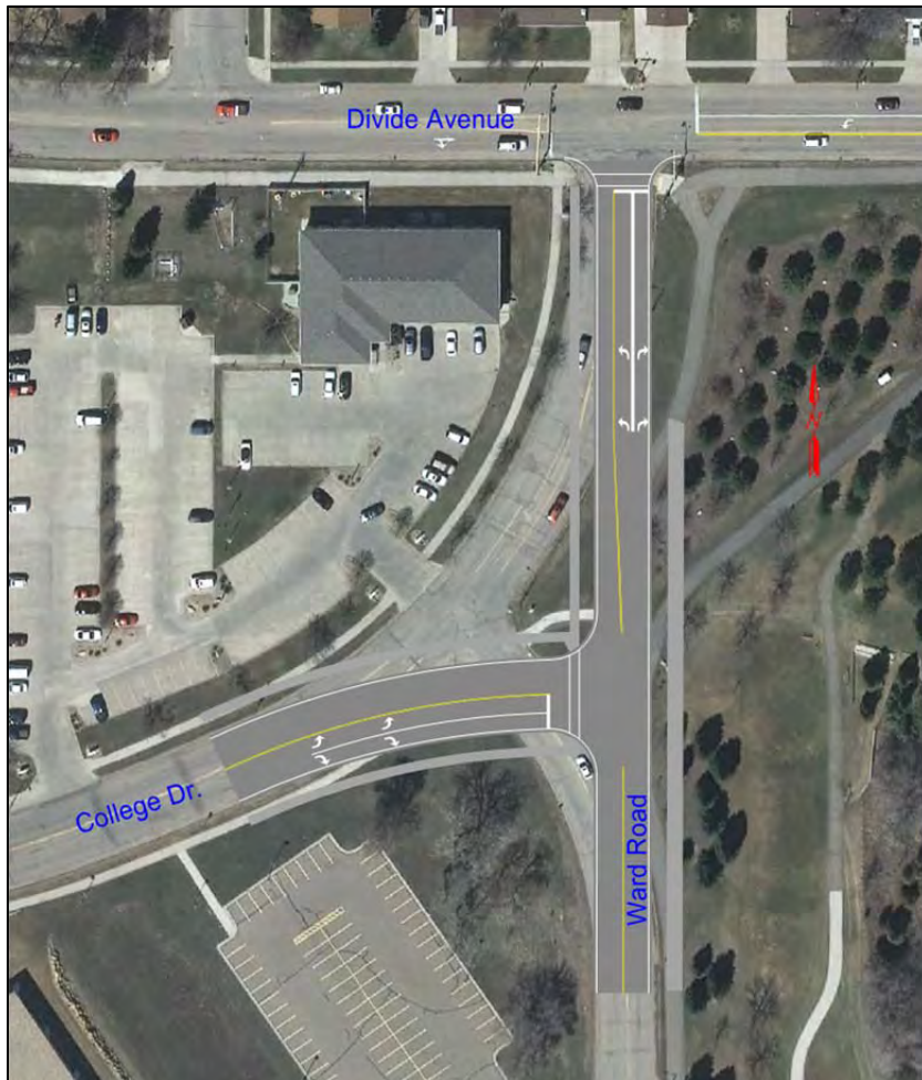
Figure 46. Ward Road Realignment
