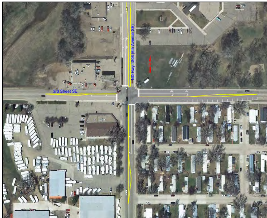
Figure 20. Lane and Curb Configuration at Intersection of ND Highway 1806 S and 3rd St
