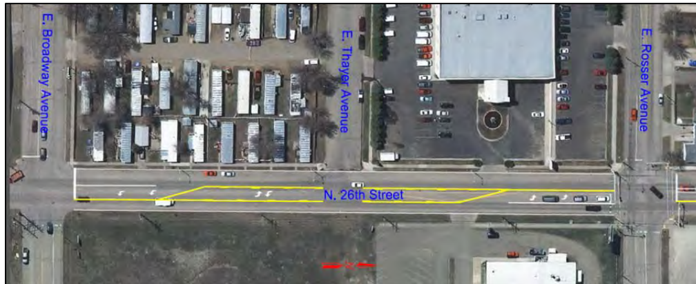
Figure 41. Example of Implementation of 3-Lane Section on 26th Street
