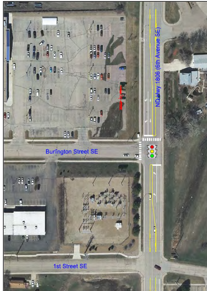
Figure 21. Turn Lanes and Possible Signal at ND 1806S and Burlington Street Intersection
