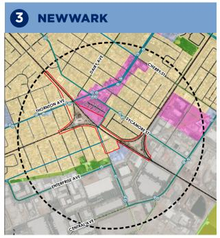
The **NEWARK STATION** study area is located where the Dumbarton Rail Corridor connects with the Coast Subdivision and Centerville lines. A station at this location would require re-alignment of existing tracks, and rail configurations and limited right-of-way space is a challenge.
