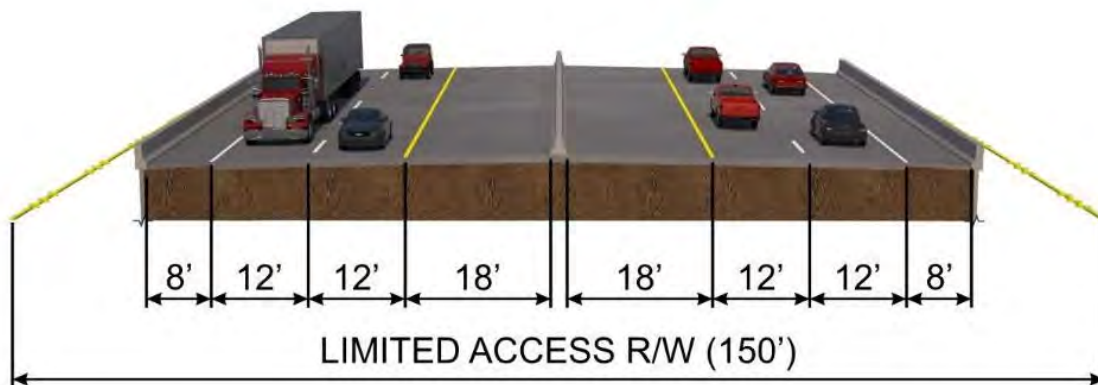
Figure 1.2. Existing Typical Section
