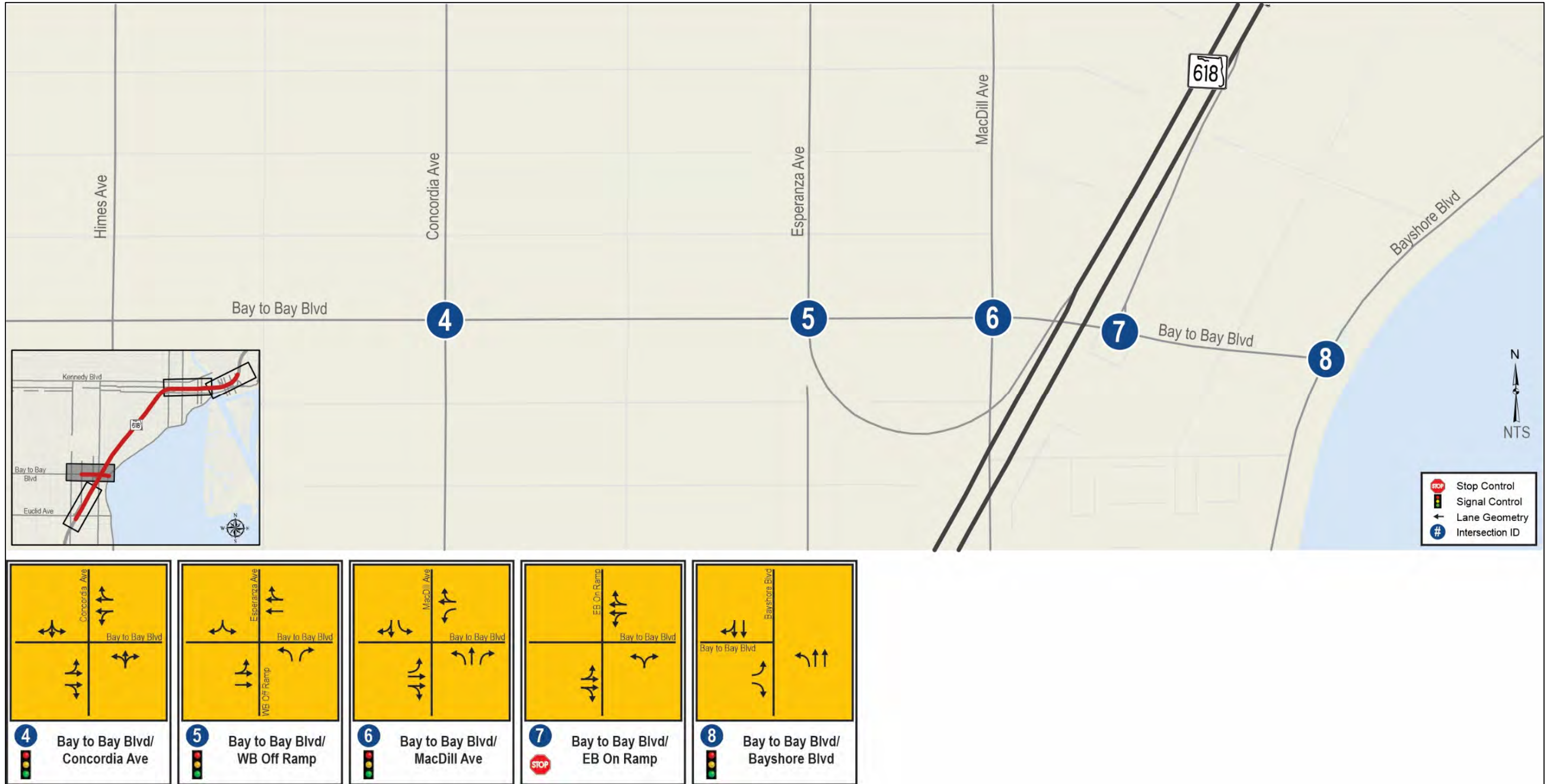
Figure 2.1 (Continued). Existing Year (2019) Lane Geometry
